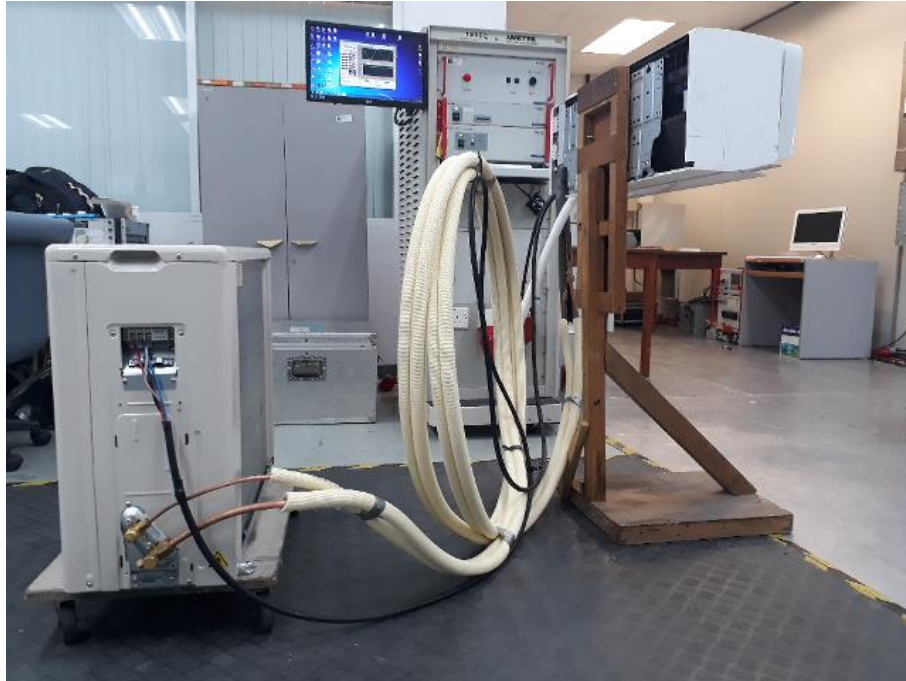
Figure AIV.3- Harmonic Current Emission and Voltage Fluctuation and Flicker test set-up
