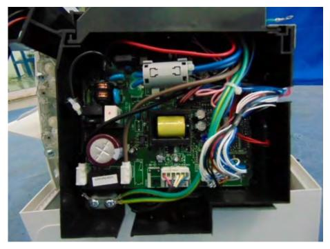
Picture No.12: PCB. compartment of indoor unit: RAS-10PKVPG-E
