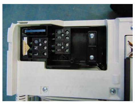
Picture No.11: Terminal view of indoor unit model: RAS-10PKVPG-E
