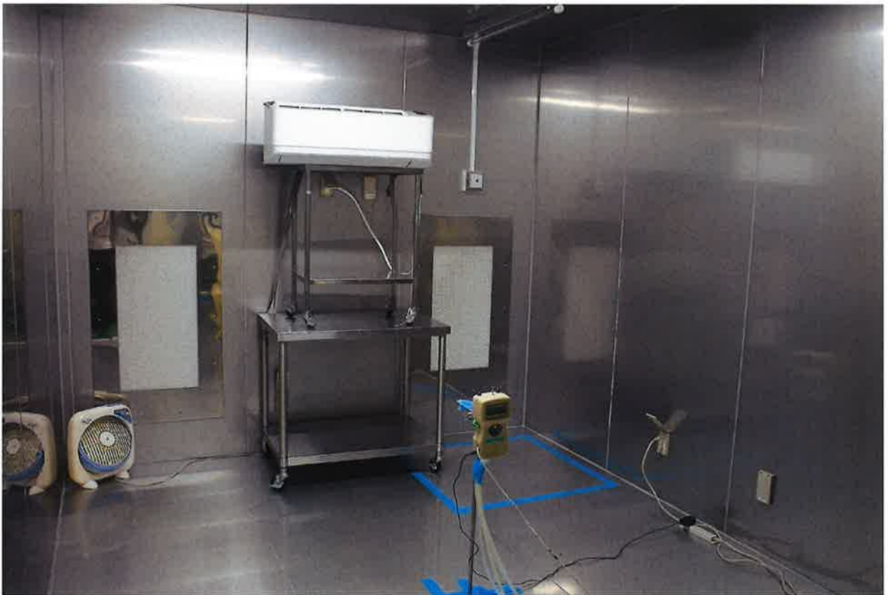
Photo 4. 25 m 3 Test chamber (Room air conditioner B)
