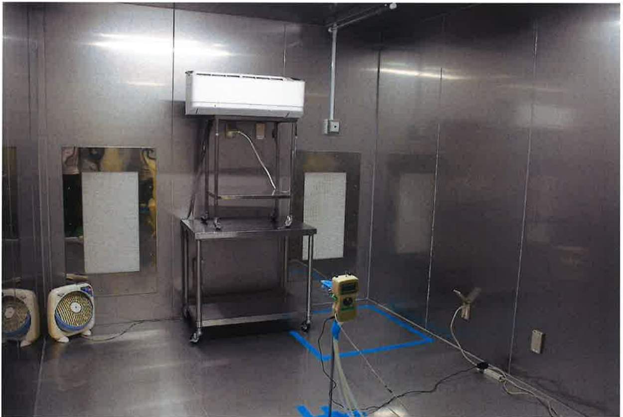
Photo 4. 25 m 3 Test chamber (Room air conditioner B)
