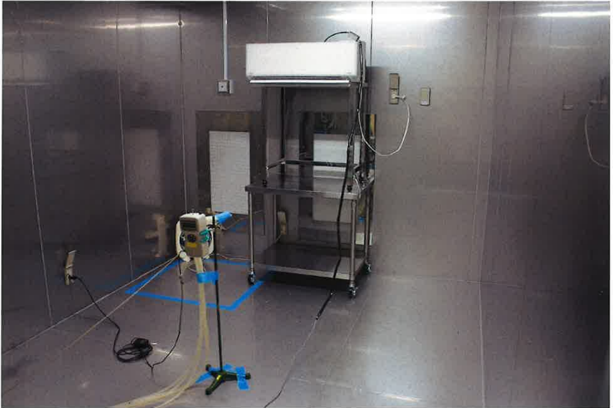
Photo 3. 25 m 3 Test chamber (Room air conditioner A)
