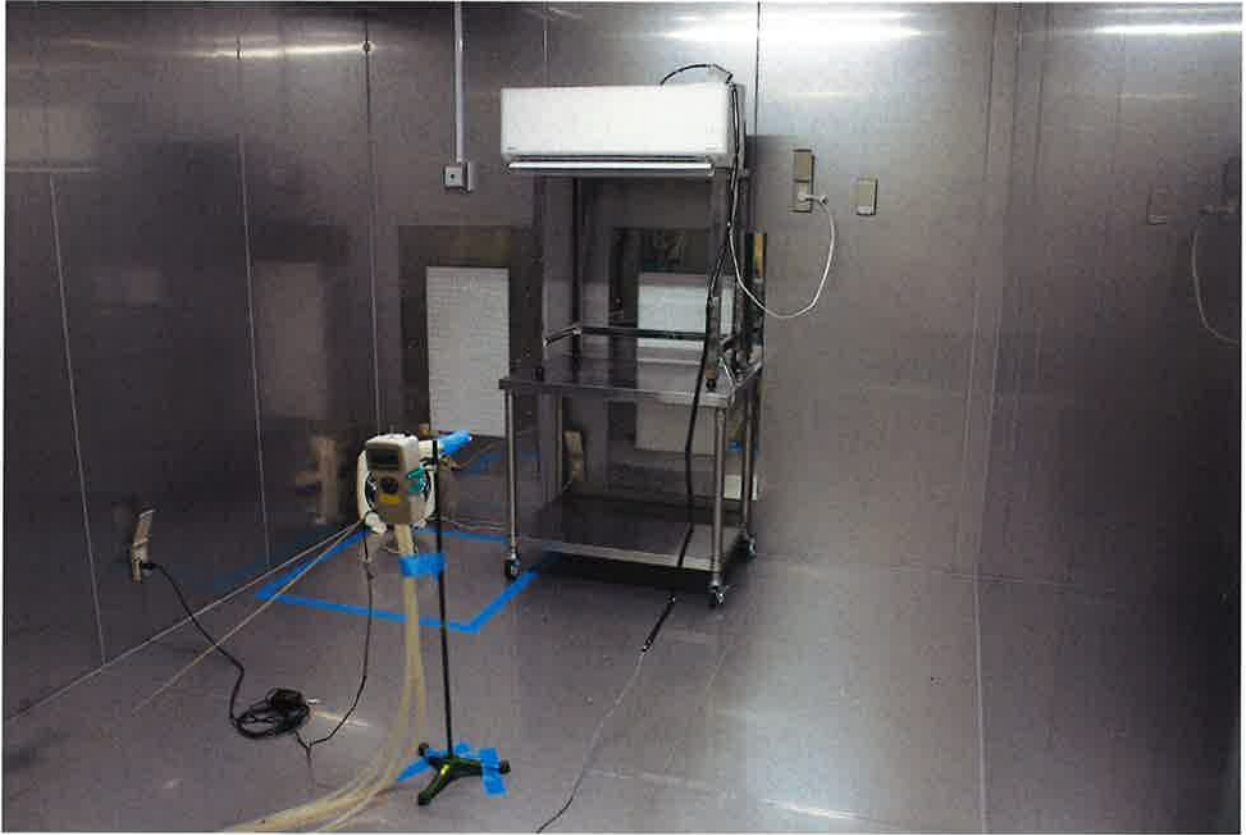
Photo 3. 25 m 3 Test chamber (Room air conditioner A)
