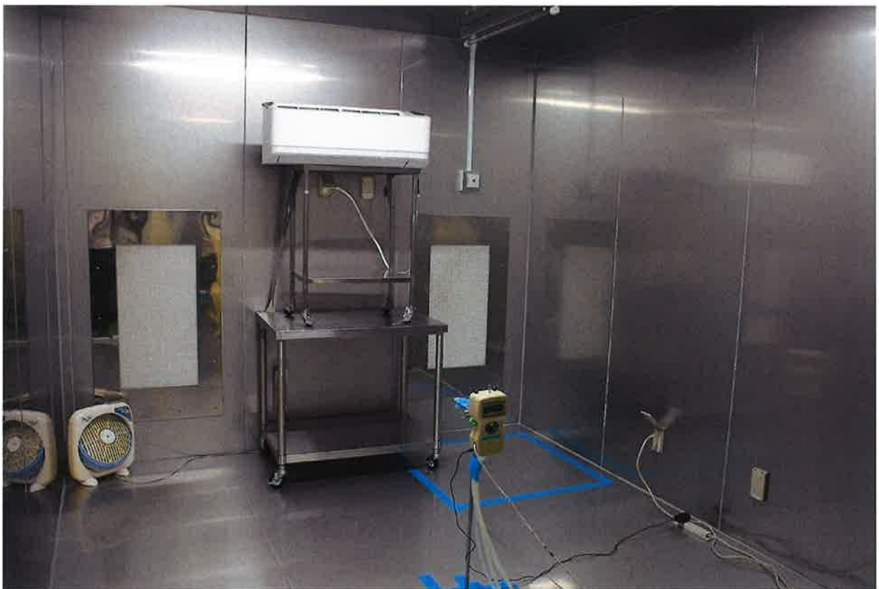
Photo 4. 25 m 3 Test chamber (Room air conditioner B)
