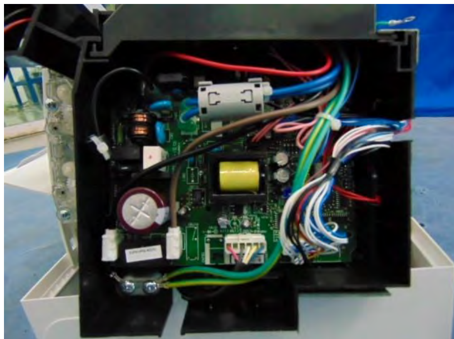
Picture No.12 : PCB. compartment of indoor unit: RAS-16PKVPG-E
