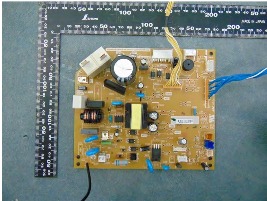
Picture No.70: Component view of PCB model: WP-048
