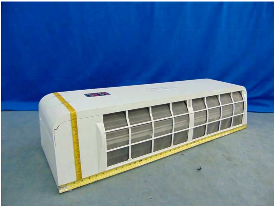
Picture No.61: Overall view of indoor unit model: RAS-24PKVSG-EE
