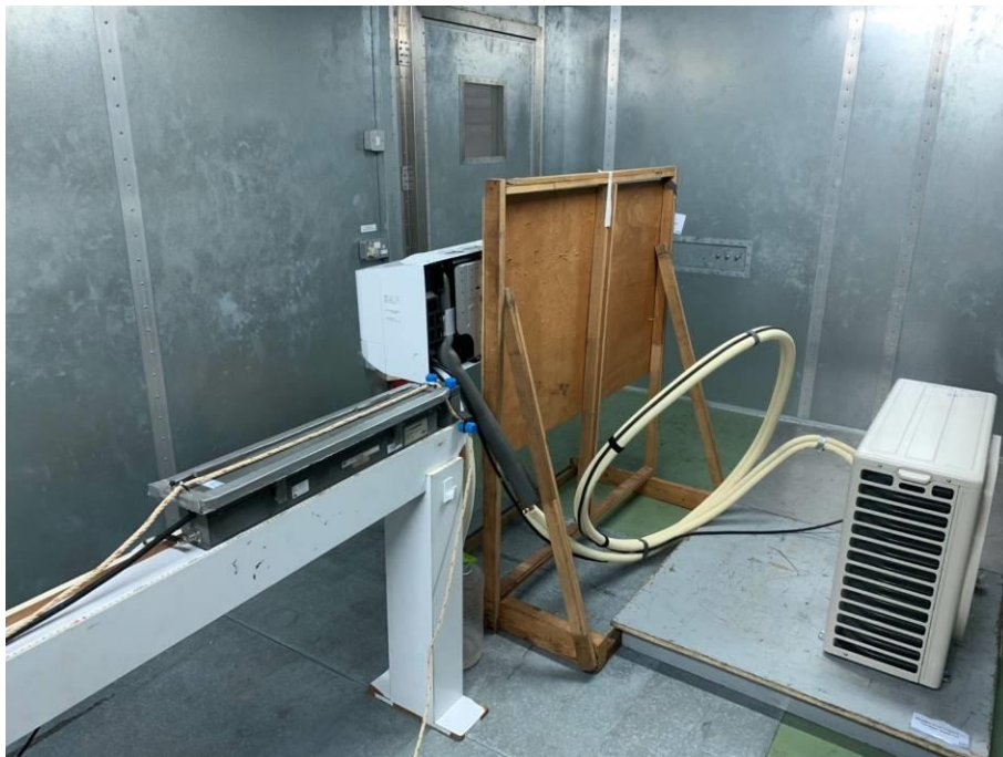
Figure AIV.2: Continuous Disturbance Power test set-up
