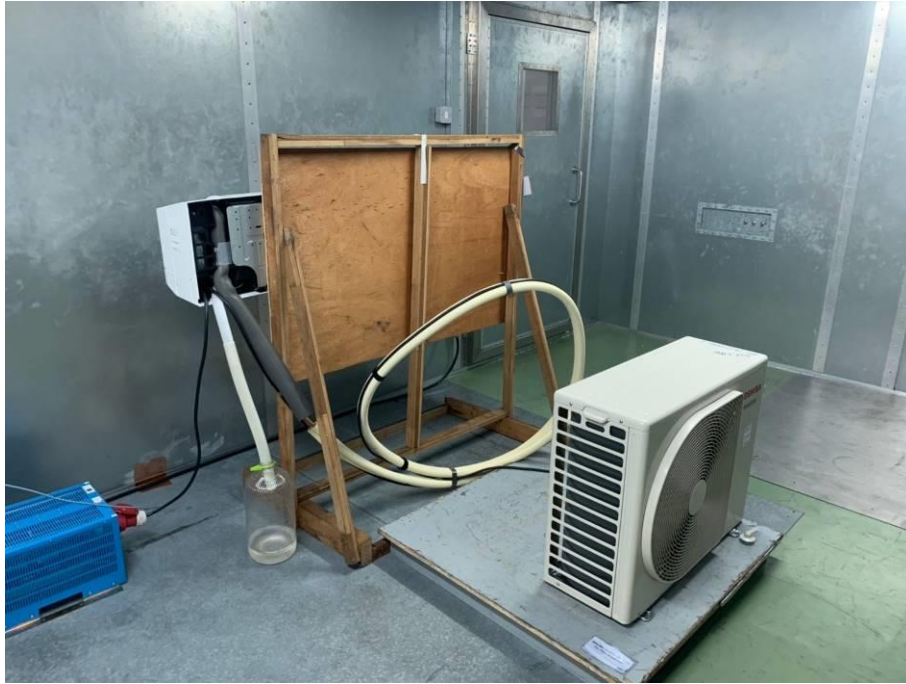
Figure AIV.1: Mains Terminal Continuous/Discontinuous Disturbance Voltage test set-up
