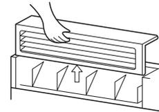
**3 Lift up the air discharge and remove it.**
