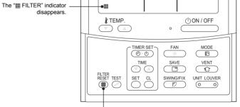
When the cleaning is complete, push the "FILTER RESET" button.
