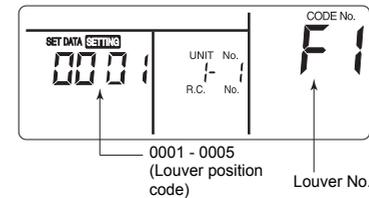
\* F1 appears in the CODE No. section on the remote controller. This indicates that the louver 01 shown in the following figure is selected.
